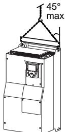
ALTIVAR 71 drives up to ratings ATV71HD15M3X and ATV71HD18N4 can be removed from their packaging and installed without a handling device.
